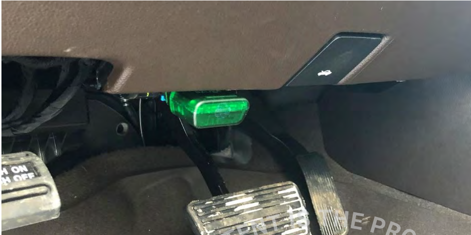
Figure 4-3: Azuga Plug-In Device Installed in OBD-II Port
