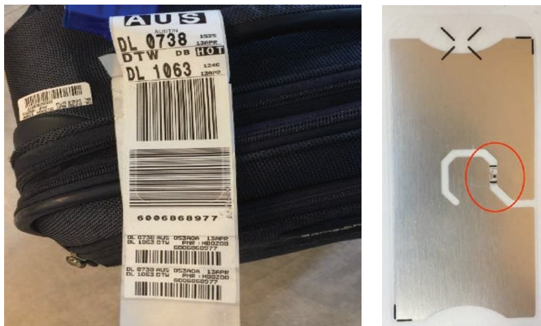
Figure 4. Example of an RFID tag: a Delta baggage tag (left) and the RFID tag embedded in it (right).
