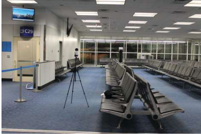
Figure 6-4. Gate hold area with acoustical ceiling tile and carpet.
