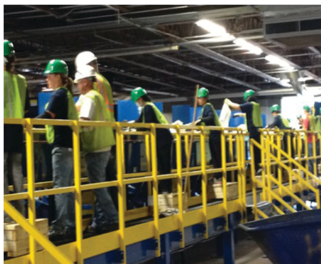
FIGURE 7 Workers at CLT’s Recycling Center sort waste through a conveyor operation (Source: Charlotte–Douglas International Airport).
