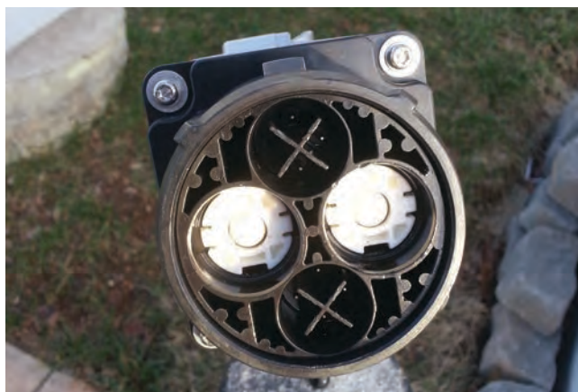
FIGURE 5 Level 3 connectors: (Left) CHAdemo connector; (Right) Tesla Supercharger. Note: The SAE combo connector, a third type of Level 3 connector, is not shown. (Source: LeighFisher January 2014.)
