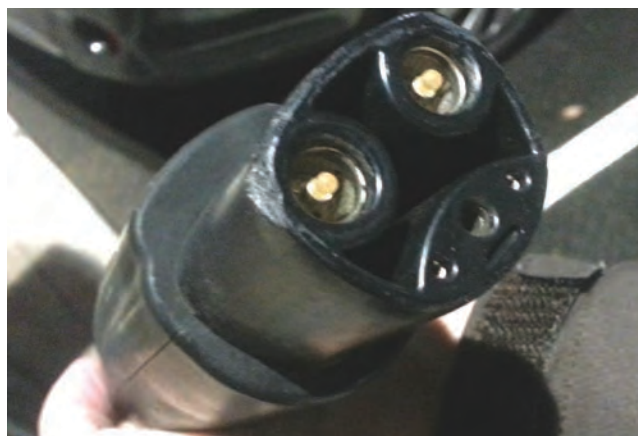
FIGURE 5 Level 3 connectors: (Left) CHAdemo connector; (Right) Tesla Supercharger. Note: The SAE combo connector, a third type of Level 3 connector, is not shown. (Source: LeighFisher January 2014.)
