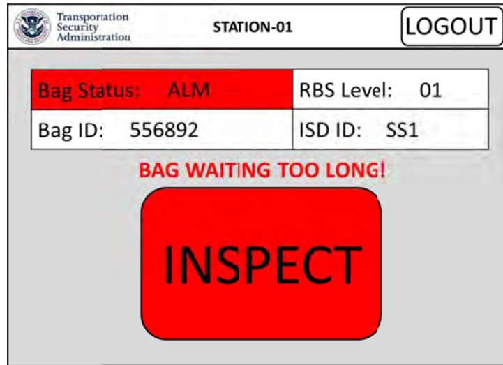
Figure 9-23 EXAMPLE OF BAG WAITING ALERT FOR ALARM BAG SCREEN
