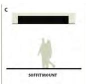
Shall be mounted perpendicular to pedestrian traffic flow
