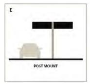
Shall be mounted perpendicular to vehicular traffic flow
