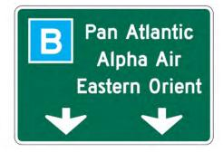
Figure 3.6. Color coding example from the 2009 MUTCD Figure 2D-1.
