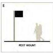
Shall be mounted perpendicular to pedestrian traffic flow
