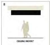
Shall be mounted perpendicular to pedestrian traffic flow
