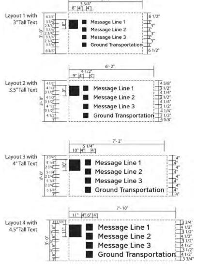
Figure 6.3. The above graphic is an example of a typical sign grid study of how different letter heights affect the overall sign grid as the size and proportions change. Note that "Ground Transportation" is used to represent the longest line length.
