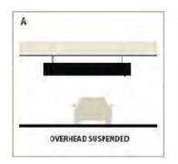
Shall be mounted perpendicular to vehicular traffic flow
