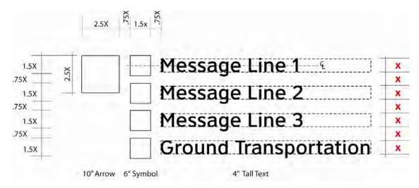
Figure 6.40. Relational spacing within a sign grid with multiple messages, symbols and arrow. Note: When designing the sign grid take into account the longest line length of any given message. In the example above "Ground Transportation" is used to calculate the longest line length.
