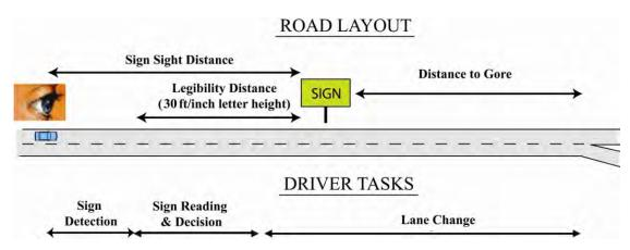
Figure 3.8. Stages of mental processing and reaction to road signs that illustrate MUTCD section 2A.13.
