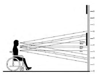
Figure 6.62. The mounting heights of a seated person and users in wheelchairs, with respect to the 10° viewing angle from the line of sight.
