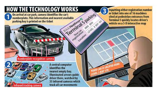
Figure 4.20. An explanation as to how technology is used to aid patrons in finding available parking and locating their vehicles at a later time.
