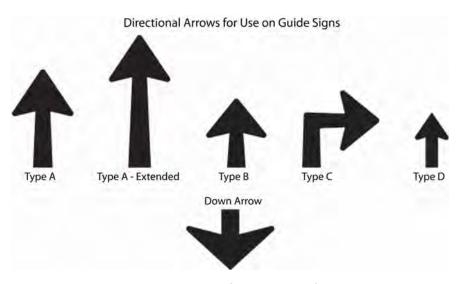
Figure 3.4. Typical arrow shapes from MUTCD figure 2D-2.
