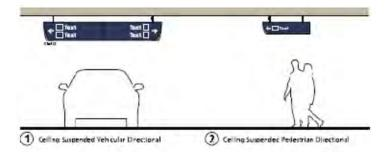
The sign system concept for parking at SJC illustrates how the pedestrian directional (2) sign is subordinate to the vehicular directional (1) sign in size, scale and location.
