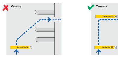
Never combine two items of routing information on one sign by using a slanted arrow (45 degrees) for continuing straight ahead for a short distance and then turning. In these cases, two signs should be used; one meaning 'straight ahead' and the other, at the decision point, for a right or left direction.
