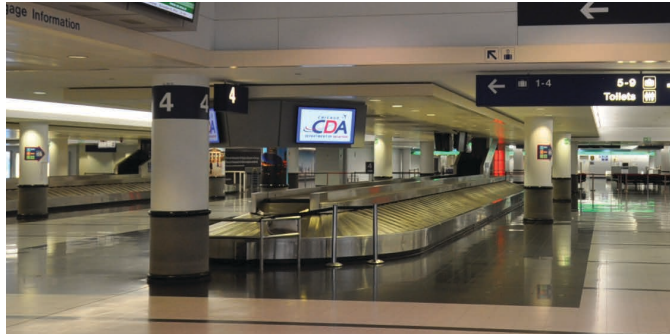
Figure 4-29. Example of a remote-fed sloped-plate baggage claim carousel at Chicago O'Hare International Airport Terminal 5.
