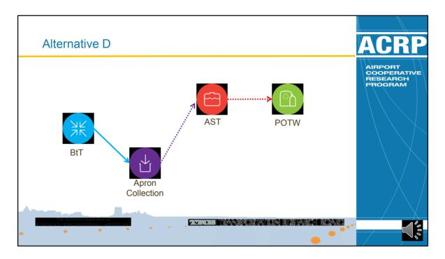
**Say:** And Alternative D where only an above ground tank is used for storage. - Blend to Temperature source controls with Apron Collection, discharge to an above ground tank and finally discharged to Publicly owned treatment works **[Click to proceed to next slide]**
