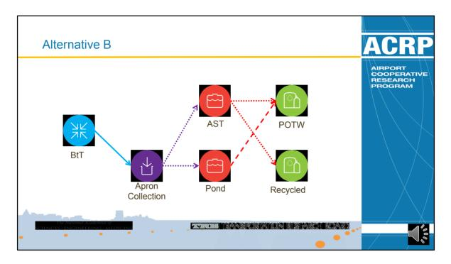
**Say:** Alternative B - Blend to Temperature treatment with Apron Collection then discharge to an Underground storage tank or Pond and finally discharged to Publicly owned treatment works or recycled
