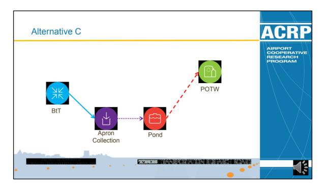
**Say:** Alternative C which is similar to Alternative B, but without the availability of recycling of concentrated runoff. - Blend to Temperature source controls with Apron Collection, discharge to a Pond and finally discharged to Publicly owned treatment works **[Click to proceed to next slide]**
