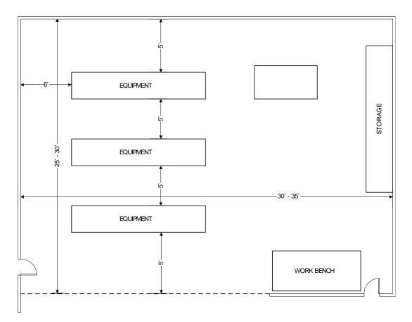
FIGURE 14. REPRESENTATIVE COMMUNICATIONS EQUIPMENT ROOM LAYOUTS
