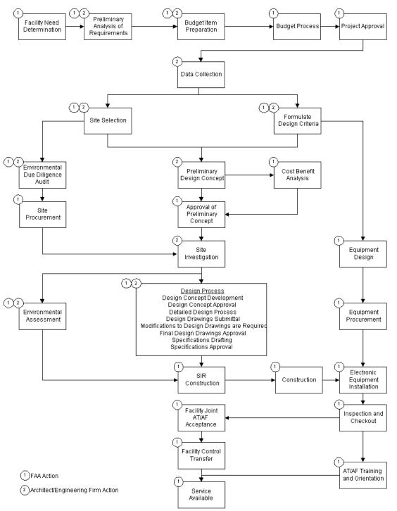
FIGURE 1-1. ATCT PLANNING AND ESTABLISHMENT PROCESS
