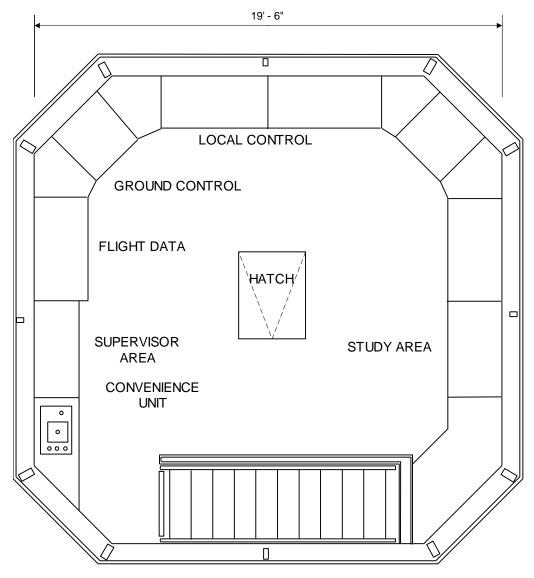
FIGURE 5. 350 SF STANDARD INTERMEDIATE ACTIVITY CONTROL CAB LAYOUT
