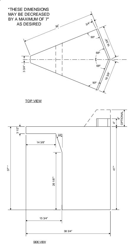
FIGURE 20. CORNER CONSOLE WITH HORIZONTAL EQUIPMENT PANEL
