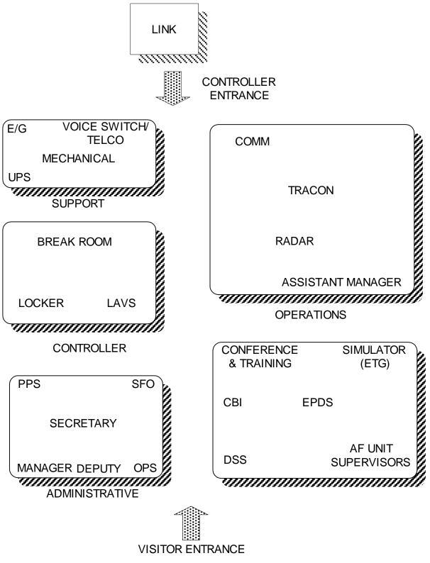
FIGURE 5-4 BLOCK DIAGRAM – ONE STORY TRACON BASE BUILDING
