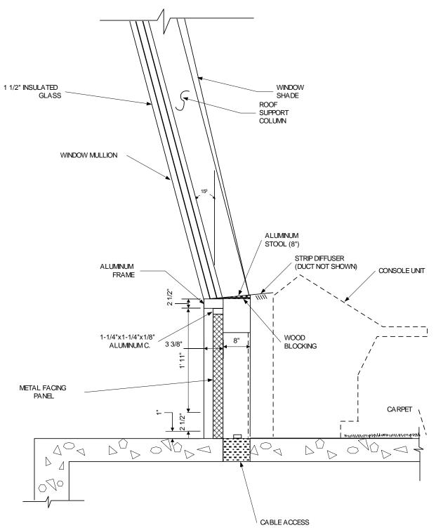
FIGURE 17. REPRESENTATIVE CAB SILL AND WALL SECTION
