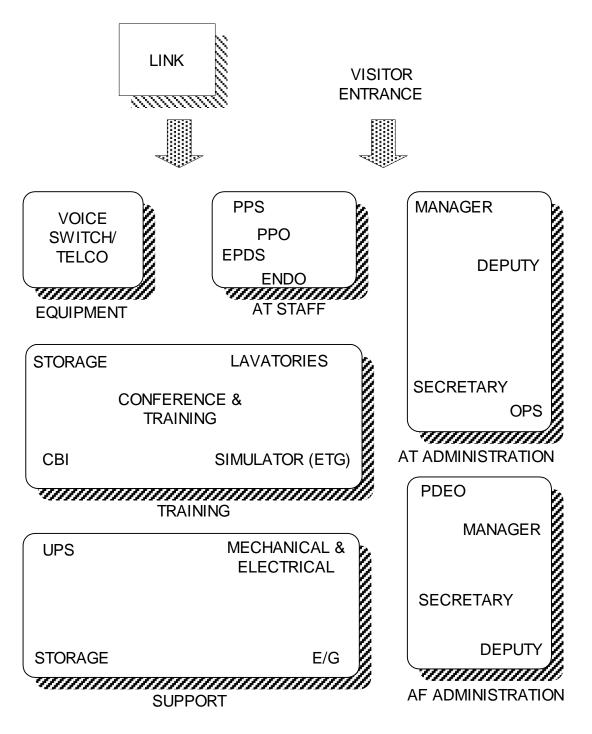
FIGURE 5-5 BLOCK DIAGRAM – TWO STORY TRACON BASE BUILDING (FIRST FLOOR )
